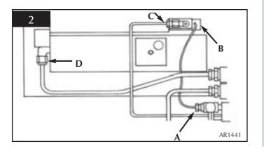
2.4 Remove the two screws at the back of the firebox and lift the burner unit clear Diagram 3
